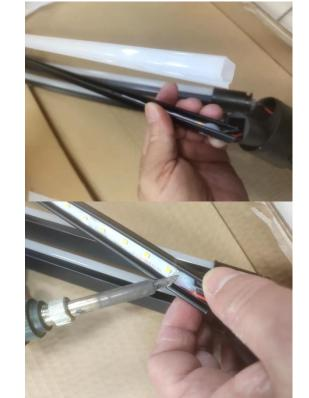
Step 3: Use an electric soldering iron to remove the wires from the circuit board, please protect the LEDs and do not touch the LEDs.
