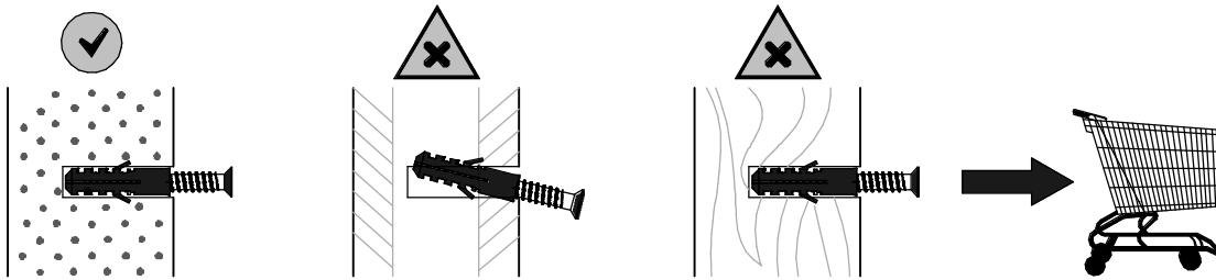
**- EN -** Before suspending or fixing furniture to the wall (in order to prevent falling over), check the type and strength of the wall. Select wall plugs and screws appropriate for the given type of the wall. In the case of doubts, contact a specialist. The installation must be performed by a competent person. **WARNING!!! If the rawlplugs with screws are attached to the product, then they are intended only for walls made of solid and homogeneous materials.**
