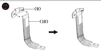
PROSIMY O OSTROŻNY MONTAŻ ELEMENTU 10, OSŁONA HARMONIJKOWA ZOSTAŁA WYKONANA Z MIĘKKIEGO TWORZYWA.
